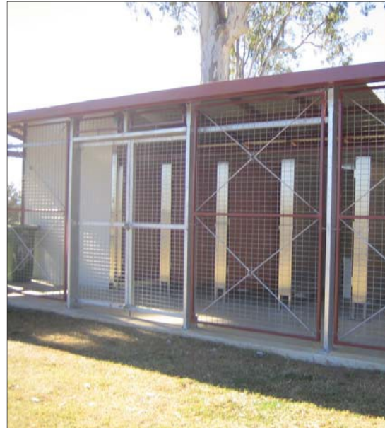
In this design, security gates are closed when the toilets are not in use but completely open during matches. Again, it is a unisex design with high visibility of all areas outside of the cubicles.
